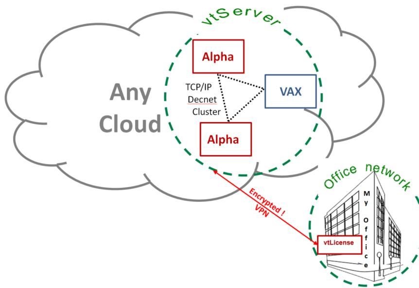
vtCloud includes a secure and transparent VPN tunnel from the Cloud provider to your office for the highest security. From the end user's perspective, there is no functional difference between vtServer emulating an Alpha system in the Cloud and vtServer emulating an Alpha system in the office. In either scenario, it is possible to create stand-alone systems and/or OpenVMS clusters, and the cluster members can be located at any Cloud provider available.
